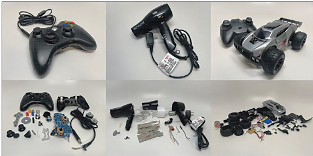
Figure 3. Original and dissected consumer products for BoilerUp Bingo. From the left, a game controller, a hair dryer and a remote-controlled car.
